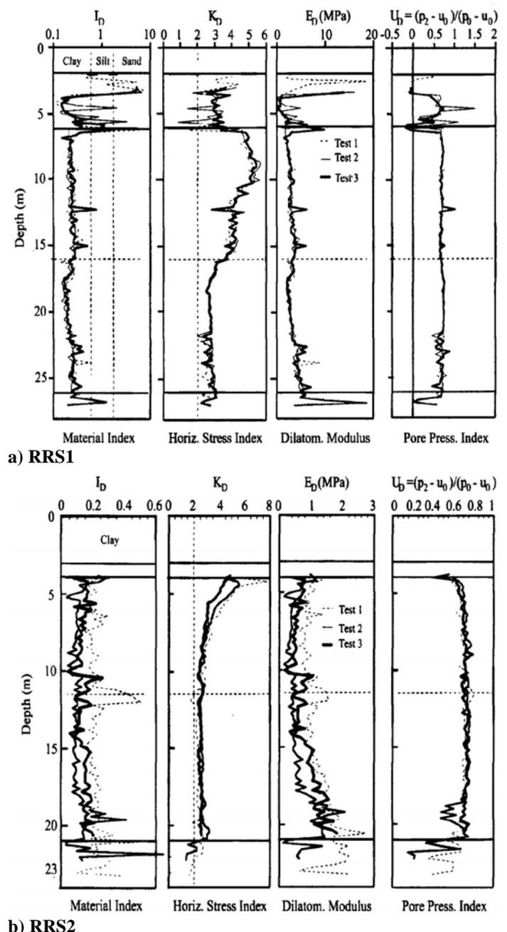
Figure 3. Dilatometer test results –  $I_D$ ,  $K_D$ ,  $E_D$ ,  $U_D$  vs Depth: (a) Research Site 1; (b) Research Site 2 (Coutinho & Oliveira, 1997; Coutinho et al., 1999).
